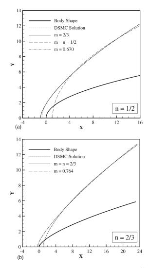
FIG. 8. Shock-wave shape curve fit on body power-law exponent of (a) 1/2, and (b) 2/3.
