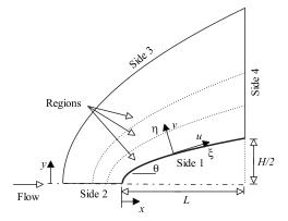
FIG. 2. Schematic view of the computational domain.
