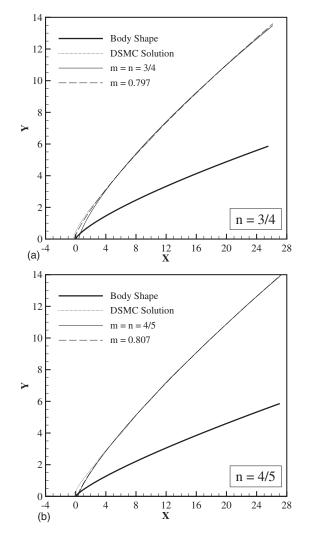
FIG. 9. Shock-wave shape curve fit on body power-law exponent of (a) 3/4 and (b) 4/5.
