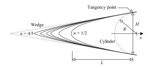
FIG. 1. Drawing illustrating the leading edge geometry.
