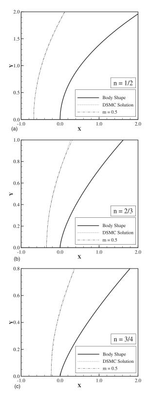
FIG. 10. Shock-wave shape curve fit, at the vicinity of the leading-edge nose, on body power-law exponent of (a) 1/2, (b) 2/3, and (c) 3/4.
