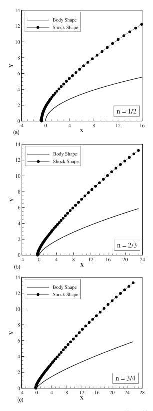
FIG. 7. Shock-wave shape on body power-law exponent of (a) 1/2, (b) 2/3, and (c) 3/4.
