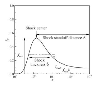
FIG. 4. Drawing illustrating the shock wave structure.
