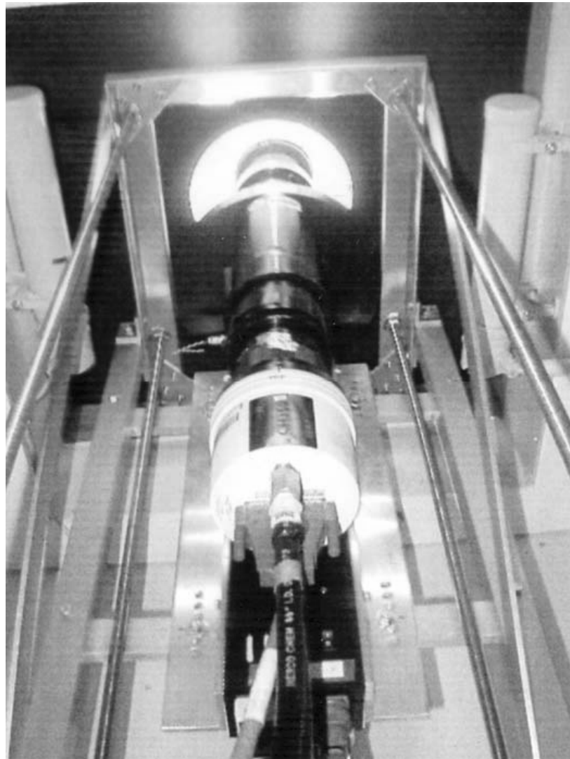
Figure 1 – All-sky, monochromatic CCD imager developed at Utah State University for imaging short-period gravity waves in the faint MLT emissions. The camera system is mounted vertically to view the night sky through a perspex dome.
