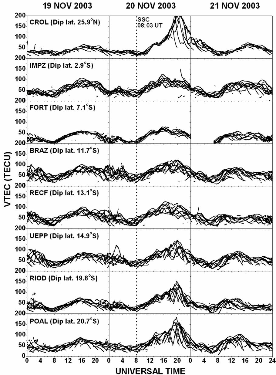
**Fig. 7.** The vertical total electron content (VTEC) variations from GPS observations (satellites above  $30^\circ$  elevation angle) at 8 receiving stations (Table 1) during the period 19 to 21 November 2003.
