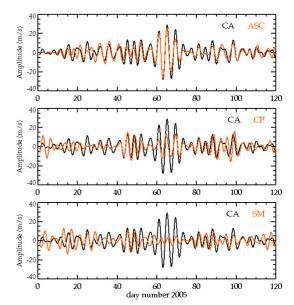
Figure 5. Amplitude and phase of 3-5 day filtered harmonic spectrum: Comparison of meteor radar zonal winds at 90 km between Cariri (CA) ( $7.4^{\circ}$  S) and Ascension (ASC) ( $7.9^{\circ}$  S) (top), Cariri and Cachoeira Paulista (CP) ( $22.7^{\circ}$  S) (middle), and Cariri and Santa Maria (SM) ( $29.7^{\circ}$  S) (bottom) during the period from January 1 to April 30, 2005. (*Fonte: GRL/AGU, 2007*)
