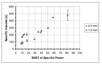
Figure 10. Isp plotted vs. the square root of specific power, xenon, 25 A.
