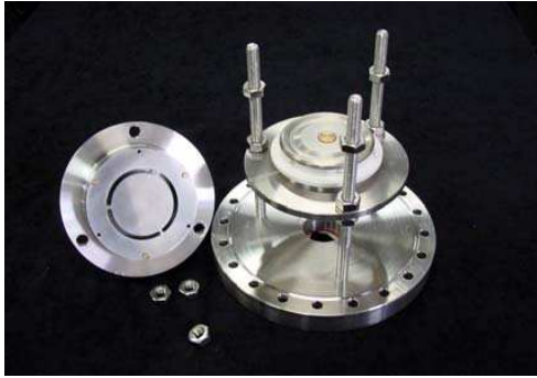
Fig. 2. Front plate of the circular cavity and gun assembly.
