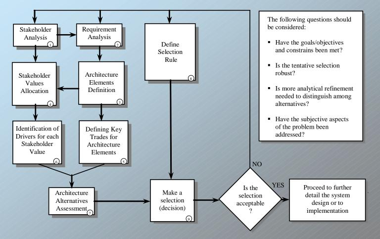
Figure 1 - Integrated space mission architecture trade off process
