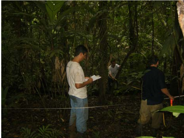
Figure 2: Field measurements, showing the tape defining the transect line, and team members measuring the perpendicular distance of each tree to that line. Field work was performed 11-23 February 2006.
