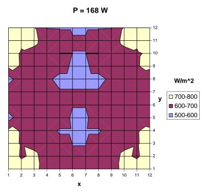
Figure 10: Absorbed Heat Radiation (W/m<sup>2</sup>) in the radiometer plate for an uncertainty of  $\pm$  83 (20:1), for lamp power P = 168W.
