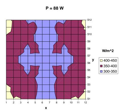
Figure 11: Absorbed Heat Radiation (W/m<sup>2</sup>) in the radiometer plate for an uncertainty of  $\pm$  42 (20:1), for lamp power P = 88 W.
