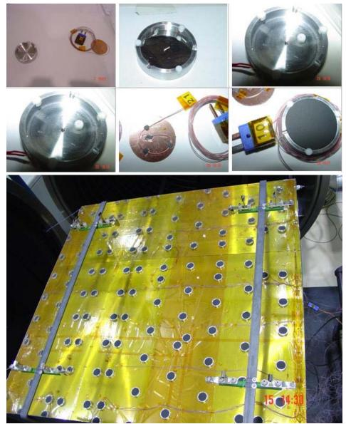
Figure 2: Bottom: view of the setup: radiometers, base plate, lamps and support. Top and middle: phases of the radiometer manufacturing process.
