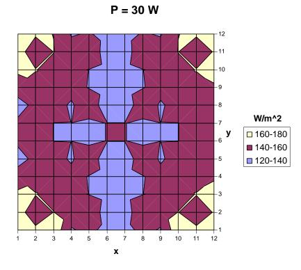
Figure 12: Absorbed Heat Radiation (W/m<sup>2</sup>) in the radiometer plate for an uncertainty of  $\pm$  19 (20:1), for lamp power P = 30 W
