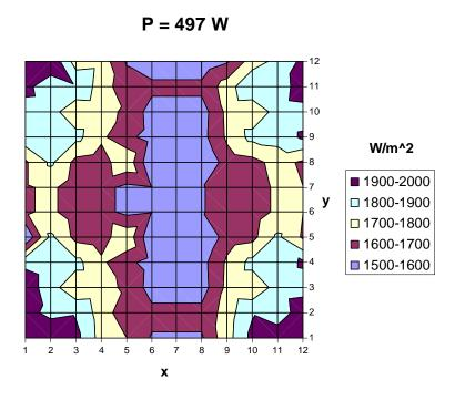
Figure 8: Absorbed Heat Radiation (W/m<sup>2</sup>) in the radiometer plate for an uncertainty of  $\pm$  177 (20:1), for lamp power P = 497W.
