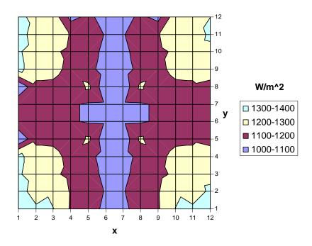
Figure 9: Absorbed Heat Radiation (W/m<sup>2</sup>) in the radiometer plate for an uncertainty of  $\pm$  119 (20:1), for lamp power P = 317W.
