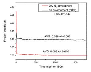
**Fig. 1a)** Evolution of the friction coefficient vs. sliding distance in air and nitrogen atmosphere.
