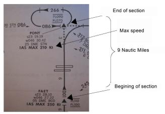
Fig. 3 Real velocity standard for air lane section velocity limits.
