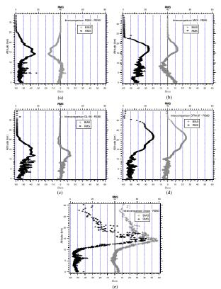
Figure 1 - Bias and RMS values for different altitude as a function of the RS80 RH values.
