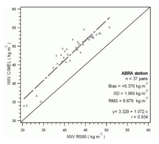
Figure 2 - Scattering diagrams of the CIMEL IWV values as function of the RS80 IWV values in ABRA station.
