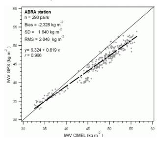
Figure 3 - Scattering diagrams of the GPS IWV values as function of the CIMEL IWV values in ABRA station.
