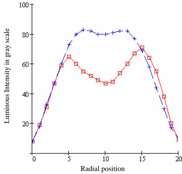
Figure 9. C<sub>2</sub> radical distribution (box, □), and soot (cross, +) at 0°.
