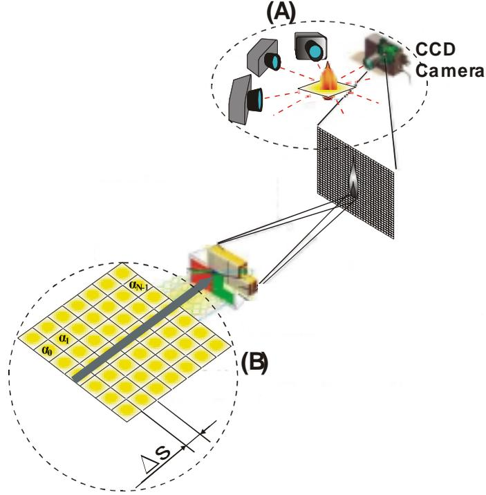
Figure 1. TC data acquisition through a RR; a) Angular CCD's cameras positions around the RR; emerging with intensity,  $I$ . The  $\alpha_i$ 's are the extinction (absorption plus scattering) linear coefficient of each layer, and  $L$  is the integration line. b) A light beam is formed within the RR.
