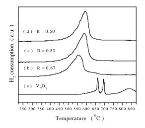
**Fig. 4.** Results of TPR profiles of (a) V<sub>2</sub>O<sub>5</sub> bulk, (b) V/Mg<sub>0.5</sub>Al, (c) V/Mg<sub>0.89</sub>Al and (d) V/Mg<sub>0.10</sub>Al. <sup>\*</sup> To whom all correspondence should be addressed. Address: Departamento de Engenharia Química de Lorena, FAENQUIL, 12600-000 Lorena, SP – Brazil E-mail: cortez@dequi.faenquil.br
