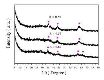
Fig. 3. XDR patterns of V-LDHs precursors calcined at 450<sup>0</sup>C, (●) MgO and (▼) MgAl<sub>2</sub>O<sub>4</sub>.
