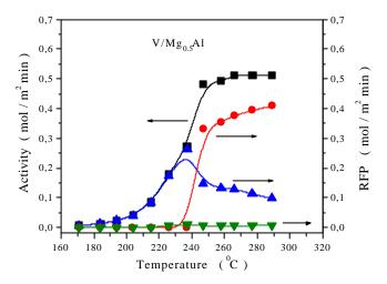
**Fig. 5.** Catalytic test of the V/Mg<sub>0.5</sub>Al catalyst in the reaction of decomposition of the isopropanol. Isopropanol ( $\blacksquare$ ) and propilen ( $\bullet$ ).
