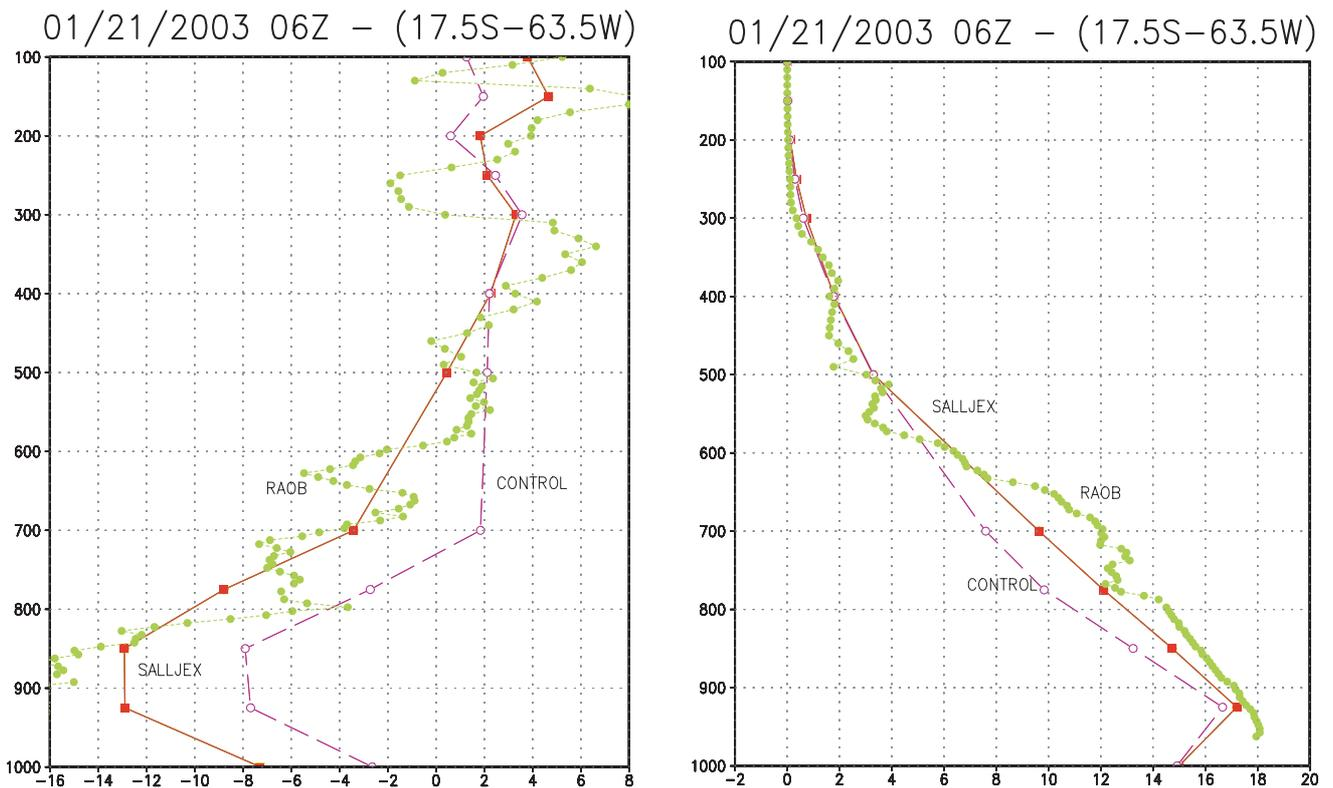
Fig.3: Vertical structure of (a) meridional wind, (b) humidity, on January, 21, from radiosonde at Santa Cruz ( 17.5°S, 63.5°W) (RAOB), forecast results using SALLJEX data and using the Control.
