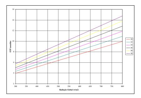
Figure 2 - Variation of the ETP with global solar radiation for different air temperature using MCA method.
