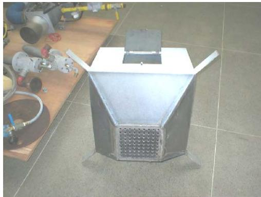
Figure 2: Front view of the combustion chamber prototype
