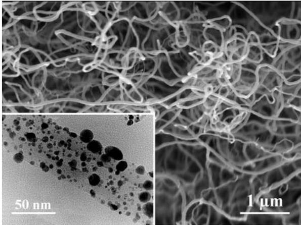
Fig 2. SEM image of carbon nanofibers. Insert: TEM image of a nanofiber covered by iridium particles
