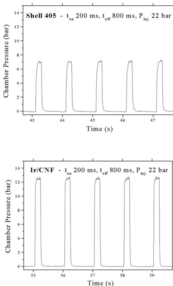
Fig. 4. Part of a chamber pressure curve of the Shell 405 (on top) and Ir/NFC (below) catalysts during a series of 100 pulses  $t_{on}$  200 ms and  $t_{off}$  800 ms.
