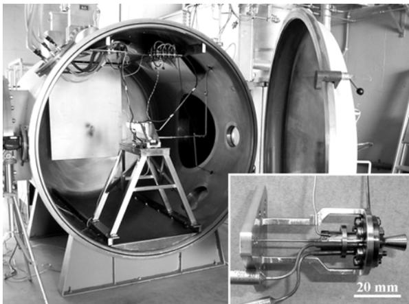
Fig. 3. Photograph of the vacuum chamber of the Test Bench of the INPE. Insert: 2 N microthruster used during the tests.
