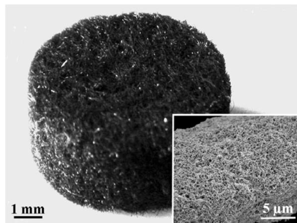
Fig. 1. Photograph of a carbon nanofiber composite. Insert: SEM image of a felt microfiber covered by carbon nanofibers.
