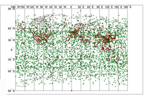
Current global coverage of instruments launched via radiosondes each day (in red) with the expected coverage from the 6 satellite COSMIC network in a 24hour period (in green) in 2005.
