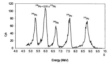
FIGURE 2 Alpha spectrum of <sup>222,220</sup>Rn progeny obtained with the electrostatic precipitator built at INPE.
