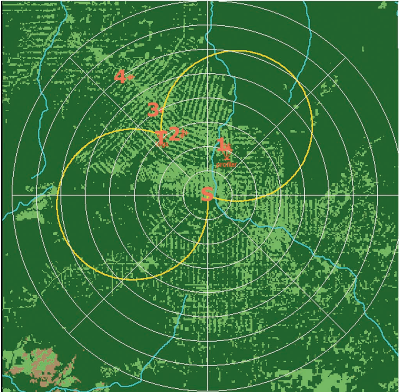
Figure 3. Deforestation in the background in light green. Dark green is forest. Rain gauge networks in red. Center of the range circles (at every 20 km) is at the S-Pol position in Fazenda Jamaica. Yellow circles are the Dual Doppler regions. TOGA radar position is indicated by T. S-Pol position is indicated by S. Rain gauge networks are indicated by numbers 1, 2, 3, and 4.
