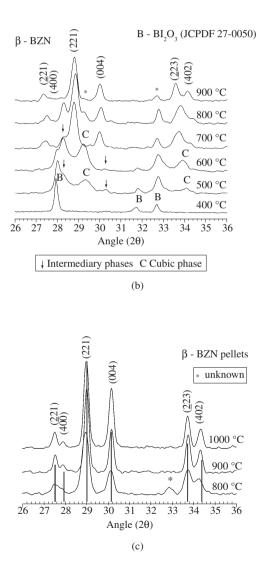
**Figure 3.** a) Extended XRD patterns of  $\beta$ -BZN powders treated for 2 hours at temperatures ranging from 500 to 900 °C; b) Zoomed 2 $\theta$  range (26-36°) for powders; c) Zoomed 2 $\theta$  range (26-36°) for pellets sintered from 800 to 1000 °C. ( $\downarrow$ ) denotes intermediary phases; and \*denotes unknown phase.
