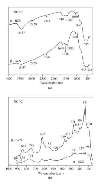
Figure 5. Spectra for  $\alpha$ - and  $\beta$ -BZN powders heated at 500 and 700 °C, respectively. a) FT-IR; and b) Raman.
