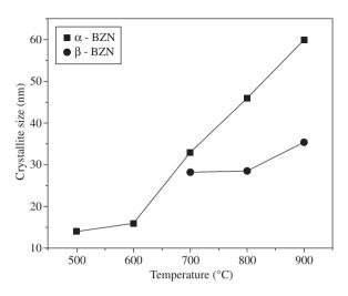
Figure 4. Crystallite size as a function of temperature for  $\alpha\mbox{-BZN}$  and  $\beta\mbox{-BZN}$  powders.
