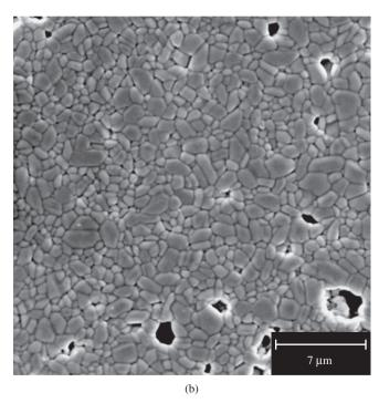
Figure 10. Microstructure observed by SEM of pellets sintered at 900 °C for 2 hours: a)  $\alpha$ -BZN; and b)  $\beta$ -BZN.
