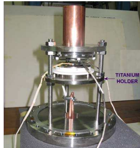
Fig. 7. Full monotron assembly with measuring thermocouples.
