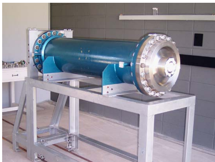
Figure 5: The new vitiated air generator (Leite, 2006).
