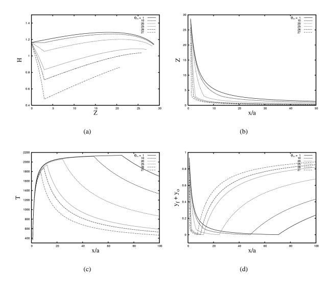
Figure 1: (a) The excess enthalpy H as function of the mixture fraction Z. (b) The mixture fraction Z as a function of the spatial coordinate x/a. (c) The temperature profile T as a function of the spatial coordinate x/a. (d) The fuel and oxidant mass fractions  $y_F$  and  $y_O$  as a function of the spatial coordinate x/a. These results were found for  $\phi_q = 0$ ,  $Z_{so} = 3$  and  $1 \le \phi_m \le 27$ .
