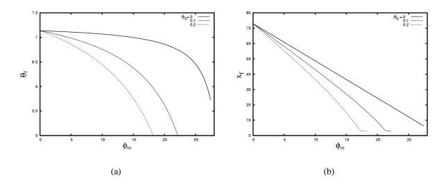
**Figure 6:** (a) Flame temperature  $\theta_f$  as a function of  $\phi_q$ . (b) Flame position  $x_f$  as a function of  $\phi_m$ . These results were found for  $\phi_q = 0$ , 0.1, 0.2 and  $Z_{so} = 3$
