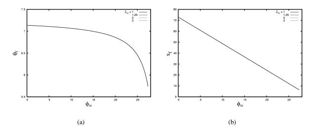
**Figure 3:** (a) Flame temperature  $\theta_f$  as a function of  $\phi_m$ . (b) Flame position  $x_f$  as a function of  $\phi_m$ . These results were found for four values of the soot zone position  $Z_{so} = 1, 1.25, 2, 3; \phi_q = 0$ .
