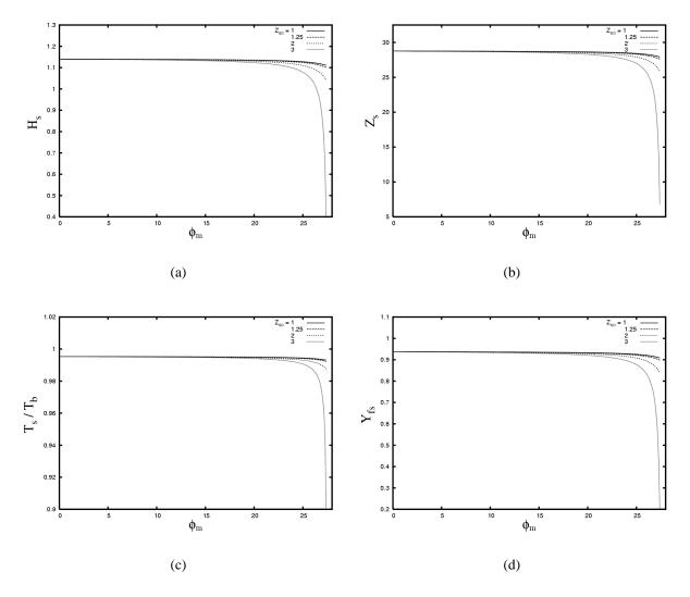
**Figure 2:** (a) Droplet surface excess enthalpy  $H_s$  as a function of the  $\phi_m$ . (b) Droplet surface mixture fraction  $Z_s$  as a function of the  $\phi_m$ . (c) Droplet surface temperature  $T_s/T_b$  as a function of the  $\phi_m$ . (d) Droplet surface fuel mass fraction  $y_{Fs}$  as a function of the  $\phi_m$ . These results were found for four values of the soot zone position  $Z_{so} = 1, 1.25, 2, 3; \phi_q = 0$ .
