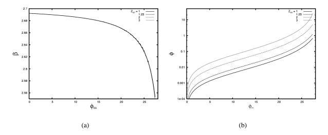
**Figure 4:** a) Vaporization constant  $\beta$  as a function of  $\phi_m$ . b) Soot mass  $\phi$  as a function of  $\phi_m$ . These results were found for four values of the soot zone position  $Z_{so} = 1, 1.25, 2, 3; \phi_q = 0$ .
