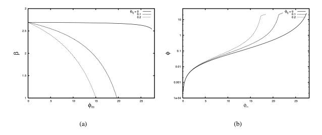
Figure 7: Vaporization constant  $\beta$  as a function of  $\phi_m$ . These results were found for four values of the soot zone position  $\phi_q = 0, 0.1, 0.2; Z_{so} = 3.$
