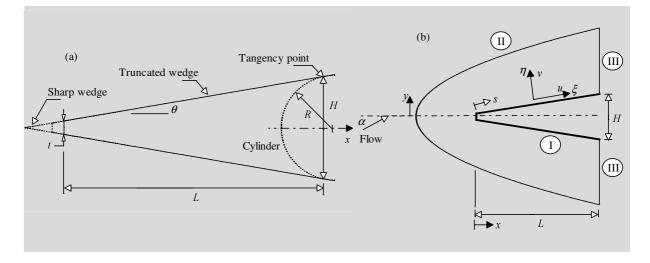
Figure 1: Drawing illustrating (a) the leading edge shapes and (b) the computational domain.
