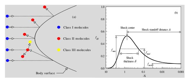
Figure 2: (a) Drawing illustrating the classification of molecules and (b) Schematic of shock wave structure.
