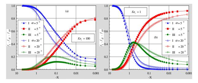
Figure 4: Distributions of molecules for classes I, II and III along the stagnation streamline parameterized by the angle of attack for thickness Knudsen number  $Kn_t$  of (a) 100 and (b) 1.
