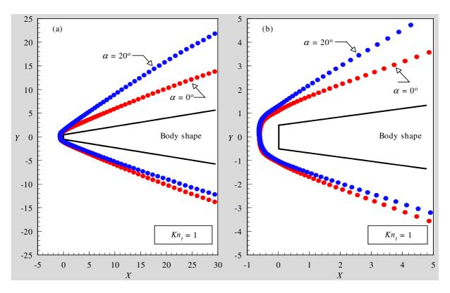
Figure 5: Shock-wave shapes on truncated wedges as a function of the angle of attack for thickness Knudsen number  $Kn_i$  of 1: (a) shock-wave on the total leading edge and (b) magnified view at the vicinity of the leading-edge nose.
