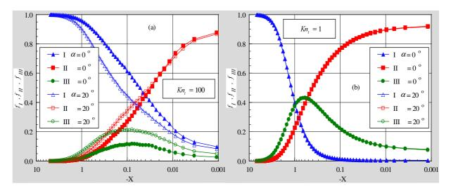
Figure 3: Distributions of molecules for classes I, II and III along the symmetry line parameterized by the angle of attack for thickness Knudsen number  $Kn_t$  of (a) 100 and (b) 1.
