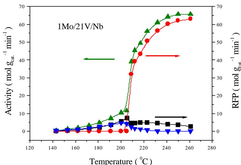
**Fig. 3.** Catalytic results for the isopropanol oxidation of 1Mo/21V/Nb catalyst versus reaction temperature. (○) Isopropanol; (●) propylene; (■) acetone and (▼) di-isopropylether.
