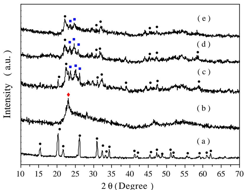
**Fig. 1.** XDR patterns of (a)  $V_2O_5$  bulk; (b)  $Nb_2O_5$ ; (c) 21V/Nb; (d) 1Mo/21V/Nb and (e) 3Mo/21V/Nb. Peaks due to ( )  $V_2O_5$  phase; (♦) TT-phase or T-phase of  $Nb_2O_5$  and ( )  $\beta-(Nb,V)_2O_5$  phase.
