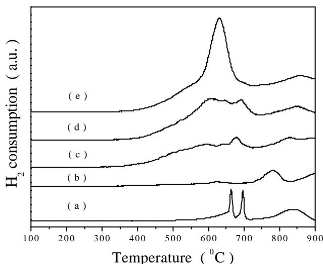
Fig. 2. TPR profiles of (a) V<sub>2</sub>O<sub>5</sub> (bulk); (b) Nb<sub>2</sub>O<sub>5</sub>; (c) 21V/Nb; (d) 1Mo/21V/Nb and (e) 3Mo/21V/Nb.
