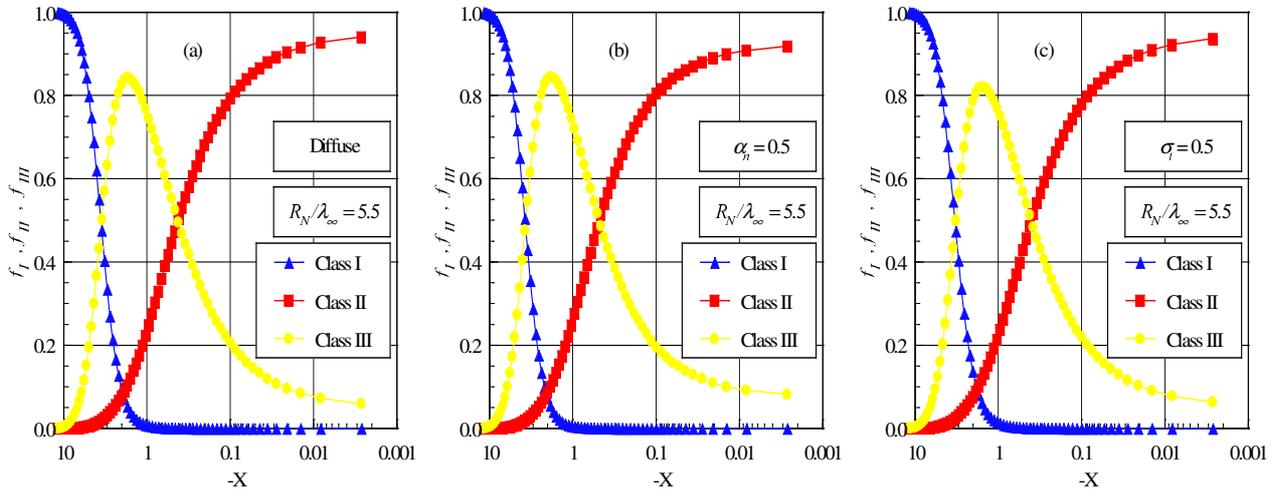
Figure 8: Distributions of molecules for classes I, II and III along the stagnation streamline for the leading edge case with  $R_N/\lambda_\infty$  of 5.5: (a) diffuse, (b)  $\alpha_n$  of 0.5 and (c)  $\sigma_t$  of 0.5.
