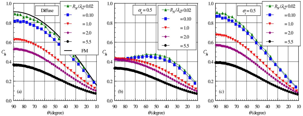
Figure 3: Distributions of the heat transfer coefficient  $C_h$  along the cylindrically portion of the round leading edges by considering (a) diffuse reflection, (b)  $\alpha_n$  of 0.5 and (c)  $\sigma_t$  of 0.5.
