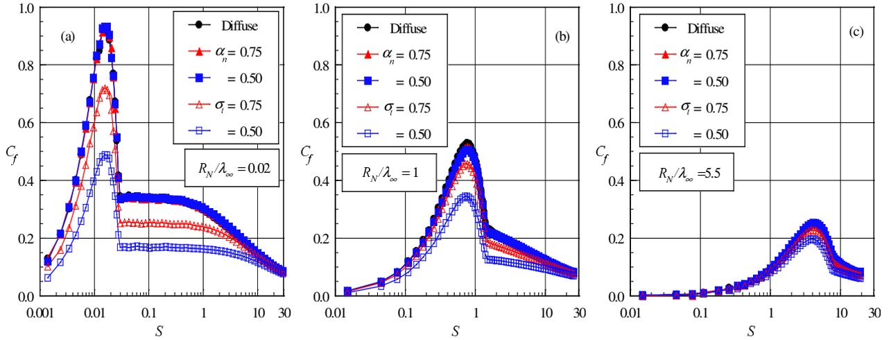
Figure 5: Distributions of skin friction coefficient  $C_d$  along the body surface as a function of the accommodation coefficient for round leading edges with  $R_N/\lambda_\infty$  (a) 0.02, (b) 1 and (c) 5.5.
