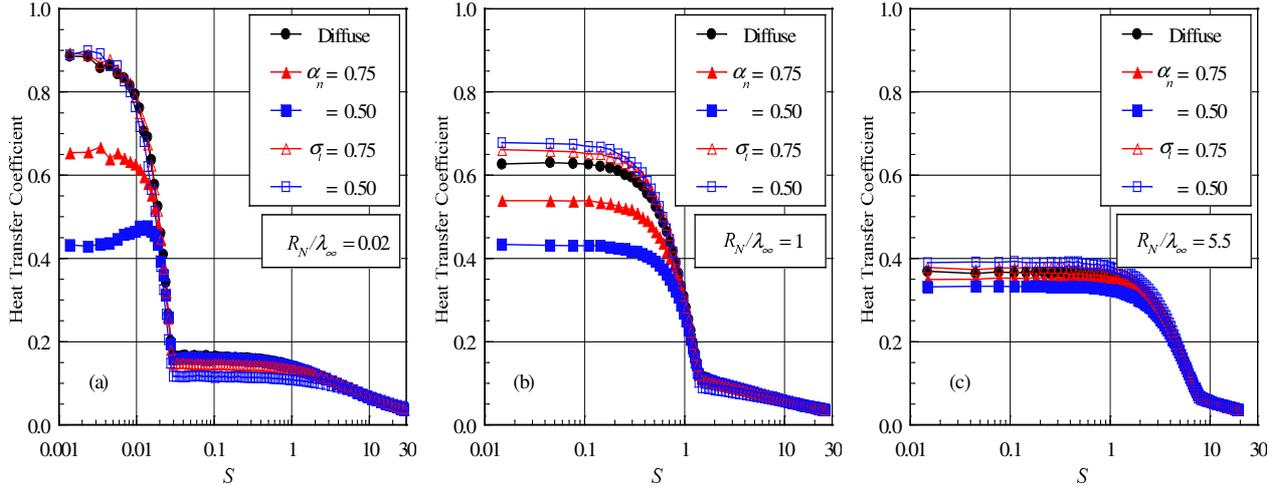
Figure 2: Distributions of the heat transfer coefficient  $C_h$  along the body surface as a function of the accommodation coefficient for round leading edges with  $R_N/\lambda_\infty$  (a) 0.02, (b) 1 and (c) 5.5.
