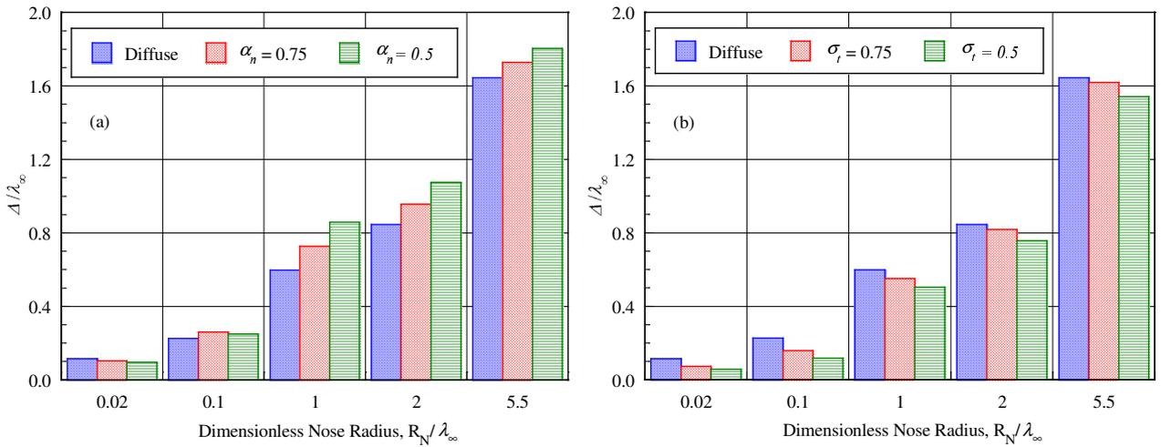
Figure 9: Dimensionless shock wave standoff distance  $\Delta/\lambda_\infty$  along the stagnation streamline for round leading edges with (a) normal and (b) tangential accommodation coefficients of 0.5, 0.75 and 1.
