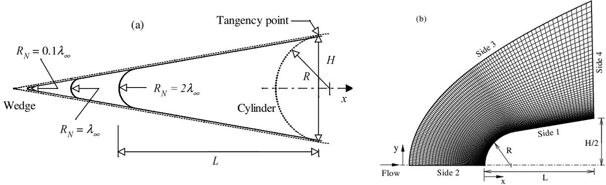
Figure 1: Drawing illustrating (a) the leading edge shapes and (b) the computational domain.
