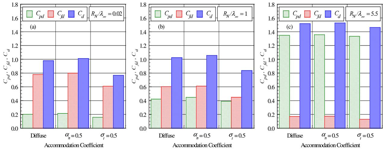
Figure 6: Pressure drag  $C_{pd}$ , skin friction drag  $C_{fd}$  and total drag coefficient  $C_d$  as a function of the accommodation coefficient for round leading edges with  $R_N/\lambda_\infty$  (a) 0.02, (b) 1 and (c) 5.5.
