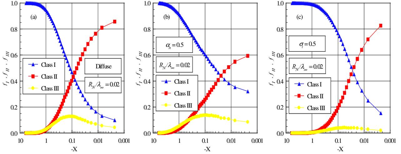
Figure 7: Distributions of molecules for classes I, II and III along the stagnation streamline for the round leading edge case with  $R_N/\lambda_\infty$  of 0.02: (a) diffuse, (b)  $\alpha_n$  of 0.5 and (c)  $\sigma_t$  of 0.5.
