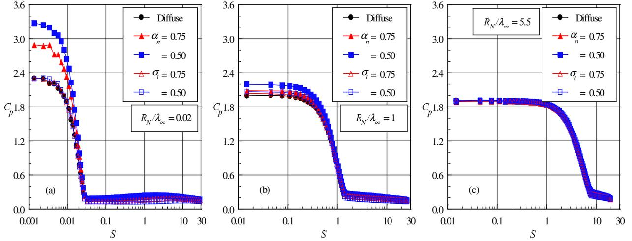
Figure 4: Distributions of pressure coefficient  $C_p$  along the body surface as a function of the accommodation coefficient for round leading edges with  $R_N/\lambda_\infty$  (a) 0.02, (b) 1 and (c) 5.5.
