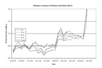
Figure 4. Variation in weight of 10-hour fuel sticks on a forest/land clearing transect at the Caiabi farm, Mato Grosso, Brazil. Fuel moisture content is calculated by the wet weight-100.
