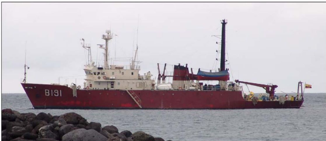
Fig. 1. The main research vessel of the INOCAR, the Orion . The Orion was constructed in 1981 and has a length of 70m and displacement of 1400 tons.
