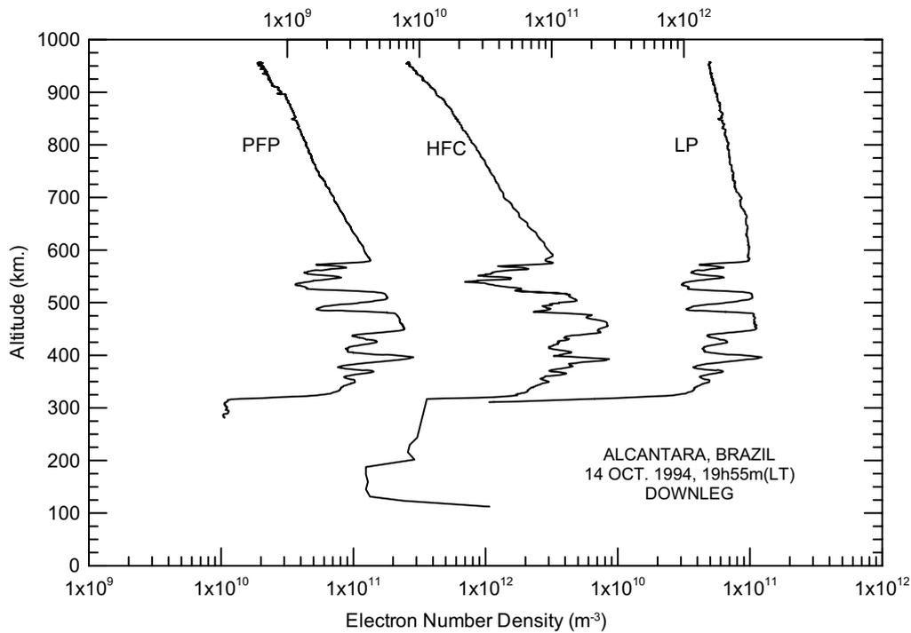
**Figure 2** – Downleg electron density profiles obtained from a Plasma Frequency Probe (PFP – bottom left scale), a High Frequency Capacitance probe (HFC – top center scale) and a Langmuir Probe (LP – bottom right scale) during the campaign Guara.
