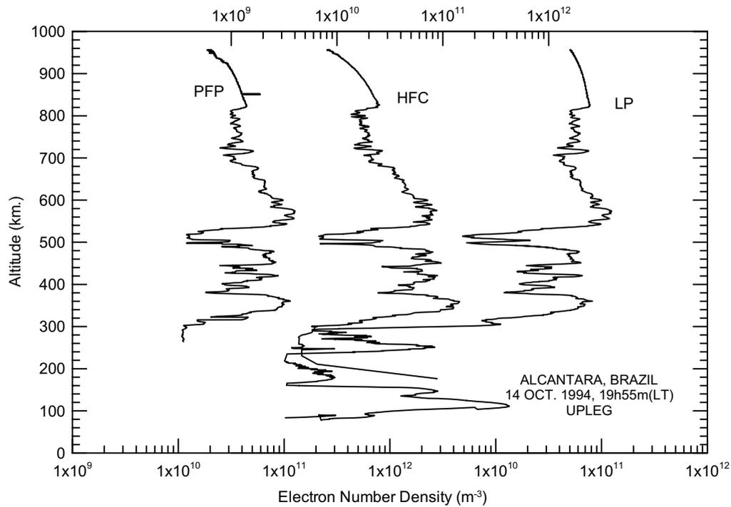
**Figure 1** – Upleg electron density profiles obtained from a Plasma Frequency Probe (PFP – bottom left scale), a High Frequency Capacitance probe (HFC – top center scale) and a Langmuir Probe (LP – bottom right scale) during the campaign Guara.
