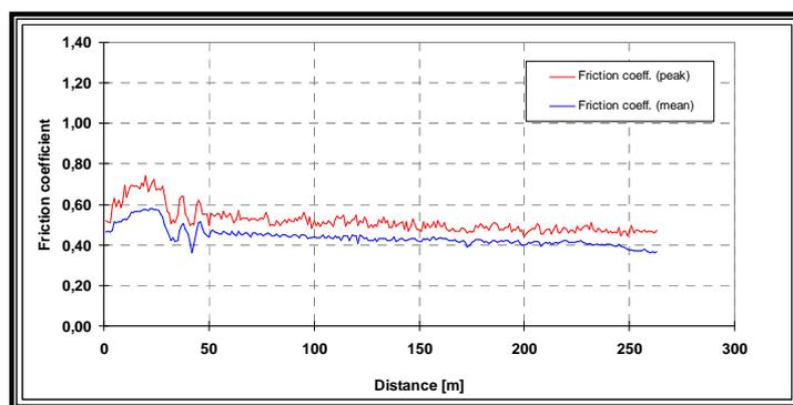
**Fig. 21a)** Evolution of the friction coefficient vs. sliding distance in UHV.
