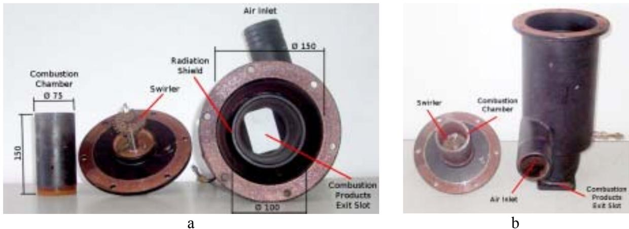
Fig. 1 – Compact combustion chamber prototype: **a** –exploded view; **b** – partial assembling
