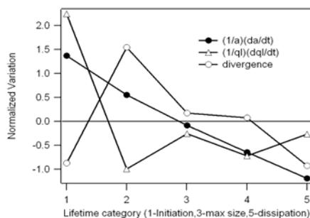
Figure 2: Average variation of the normalized area fraction for convective systems having duration between 3.5 h and 10 h, associated normalized anomalies of wind divergence and calculated condensation/evaporation rate, as function of the lifetime categories: 1 - initiation; 2 - intermediary stage between initiation and mature stage; 3 - maximum area stage (mature stage); 4 - intermediary stage between the mature and the dissipation stage; 5 - dissipation stage. Values are normalized by their
