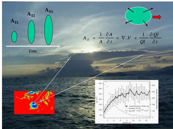
Figure 1: Schematic diagram of the convective system detection and size evolution. Figure also shows the equation relating  $A_e$ , the normalized area time rate of expansion, with the upper level wind divergence and the condensation/evaporation rate ( $Ql$  is the liquid water content). On the right side figure shows  $A_e$ , at the initiation stage, as a function of the convective system lifetime.
