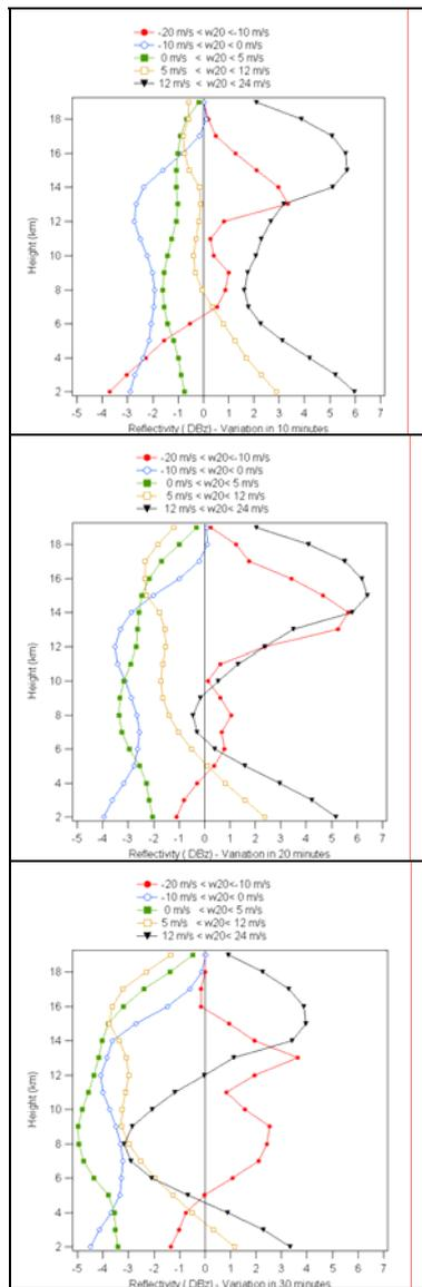
Figure 6 – Reflectivity profiles variations as function of the  $W$  value after 10 (top), 20 (middle) and 30 minutes (bottom).
