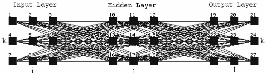
Figure 2. Architecture of a three-layer feed-forward neural network with 3x3 input/output
