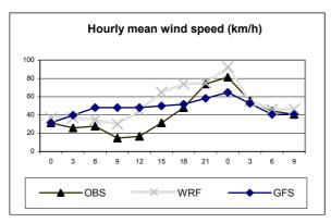
Figure 6 Observed hourly mean wind speed and models (GFS and WRF) forecast made from 00Z 23 August 2005.
