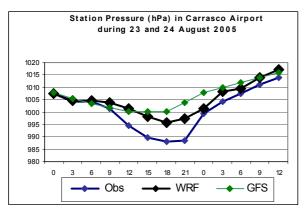
Fig 7 Station level pressure at Carrasco airport observed hourly station pressure and models (GFS and WRF) forecast between 00Z 23 August and 12Z 24 August 2005.
