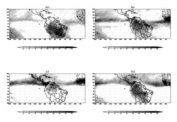
Fig. 1. Mean monthly convective cover occurrence for: (a) January, (b) April, (c) July, and (d) October. Each one were computed from the tree years 2003-2005. Value represent the number of days per month the given grid point was the infrared brightness temperature minor that 228 K.
