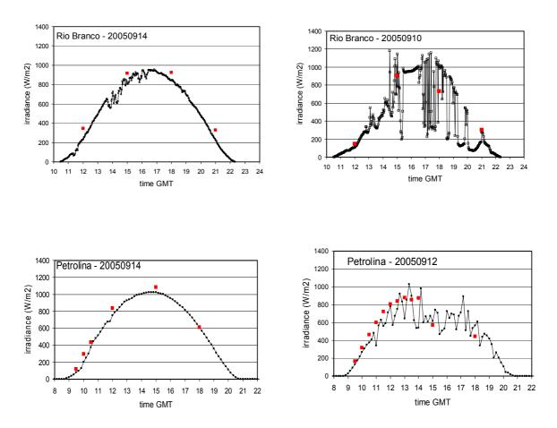
Figure 3. Daily cycles of irradiance measured by pyranometer (little black squares) and estimated by GL1.3 (red squares) in September 2005.
