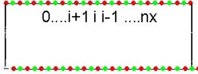
FIGURE E.1 - One dimensional staggered mesh used to calculate the scalar function \phi applied in the computation of the new magnetic field in the divergence cleaning procedure. The red dots represent the mesh grids where the magnetic field values are known and the green dots are the points where the function \phi is evaluated.
