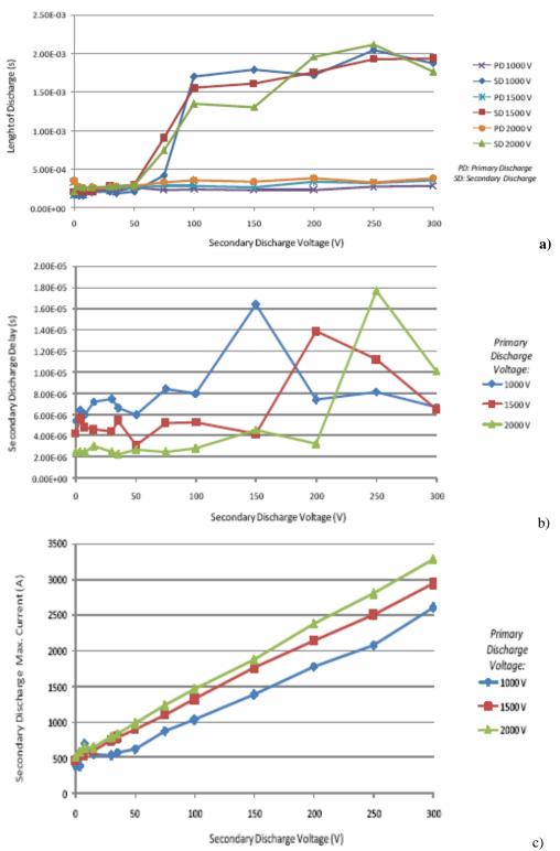
Figure 10. Length of the secondary discharge (a), delay between the first discharge and the second discharge (b) and maximum current in the secondary discharge all as function of the voltage applied in the secondary electrodes for three different primary discharge voltages.
