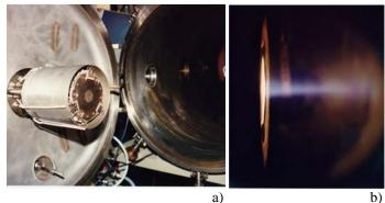
Figure 1. 7-cm ion thruster, PION-1 (a), and firing (b).
