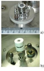
Figure 5. Rolled-tantalumoxide-foil hollow cathode: heater cartridge (a) and fully assembled (b).
