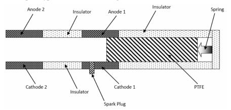
Figure 8. HFB-PPT discharge chamber.
