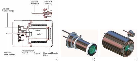
Figure 4. Schematic diagram of the 5-cm ion thruster (PION-4) (a), and both artistic conceptions of the discharge chamber with the grids (b) and the external magnetic shield (c).
